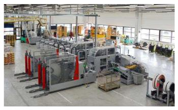
RSD inserting drum with Flystream collating systems. Including 16 JetFeeders and two feeders for preprints.
