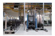
Ferag delivered a second RollSertDrum inserting drum, several MultiDisc unwinding stations for the automatic assignment of preprints and main products, and a second RollStream line with JetFeeder feeders.
